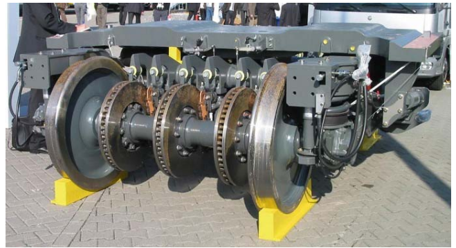
Fig. 1. Wheel-mounted ventilated brake discs used in high-speed train
