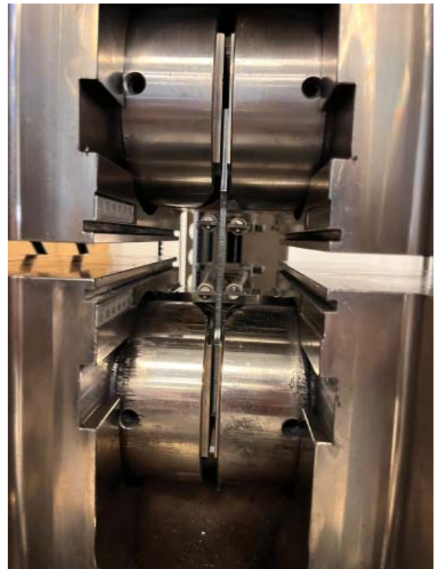
Fig. 1. Experimental tensile specimen used for calibration of the MISO model
