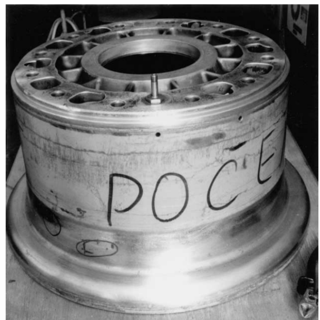
Fig. 3. The crack in the rim of an aircraft wheel
