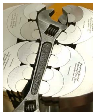
Fig. 1. Making clamping jaws of vices in the form of fractal elements
