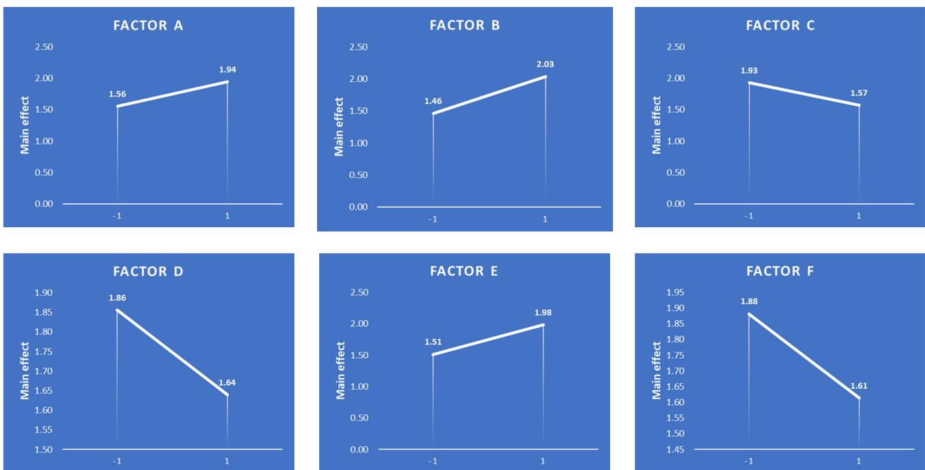
Fig. 2. Main effects plots of turning parameters on surface roughness
