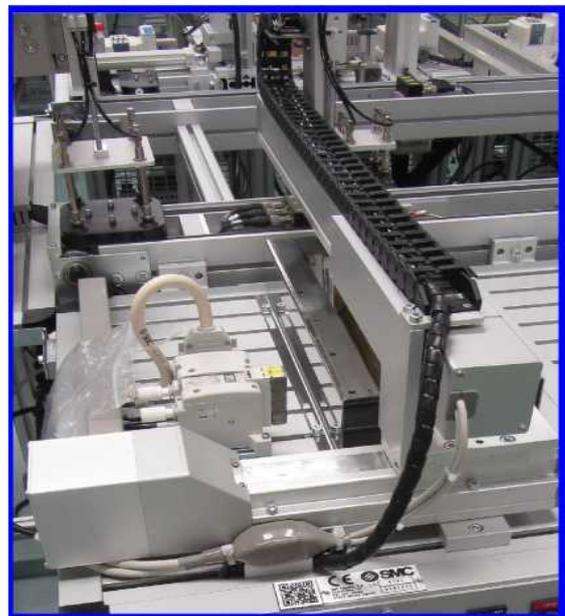
Fig. 7. Manipulators of the warehouse module
