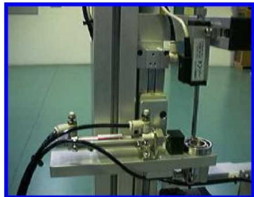
Fig. 4. Measuring manipulator
