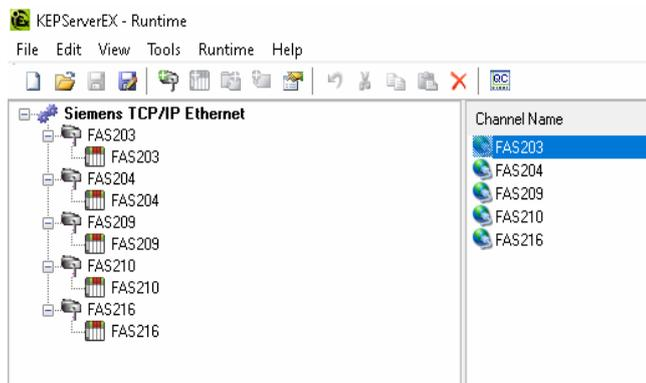
Fig. 9. Setting the modules as clients in KEPServer
