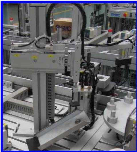
Fig. 6. Cover rejecting and transferring module
