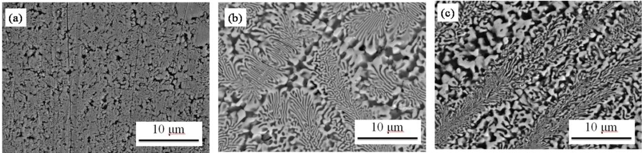
Fig. 4. SEM micrographs of the fusion zone of the samples welded with a beam power of: (a) 2400 W; (b) 2700 W; (c) 3000 W
