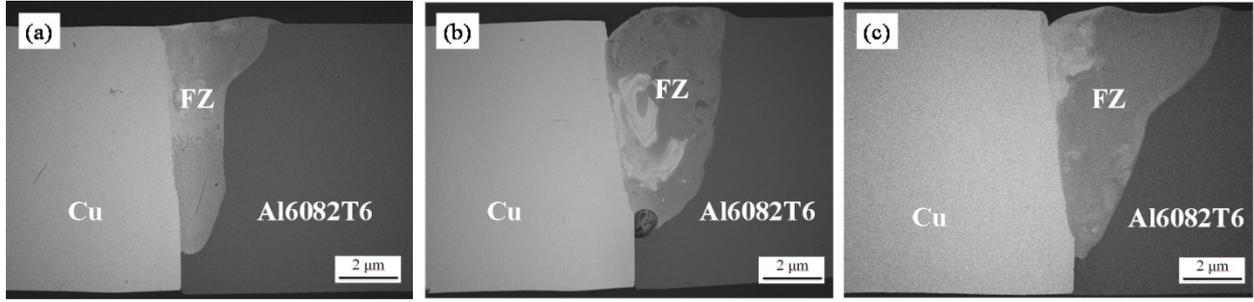
Fig. 3. Cross-sectional SEM images of: (a) sample 1 (beam power of 2400 W); (b) sample 2 (beam power of 2700 W); (c) sample 3 (beam power of 3000 W)
