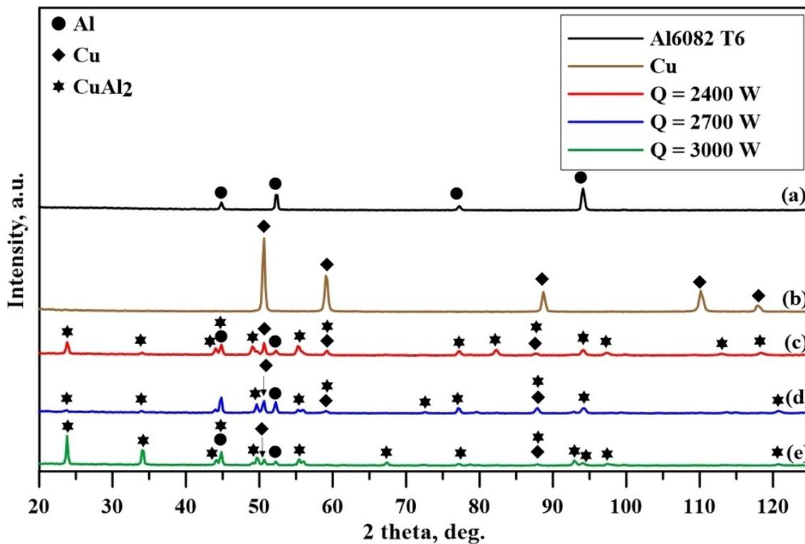
Fig. 2. X-ray diffraction patterns of: (a) Cu; (b) Al6082T6; (c) weld joint with beam power of 2400 W; (d) weld joint with beam power of 2700 W; (e) weld joint with beam power of 3000 W
