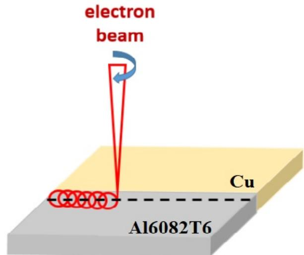
Fig. 1. Schematic of the EBW process of Cu and Al6082T6
