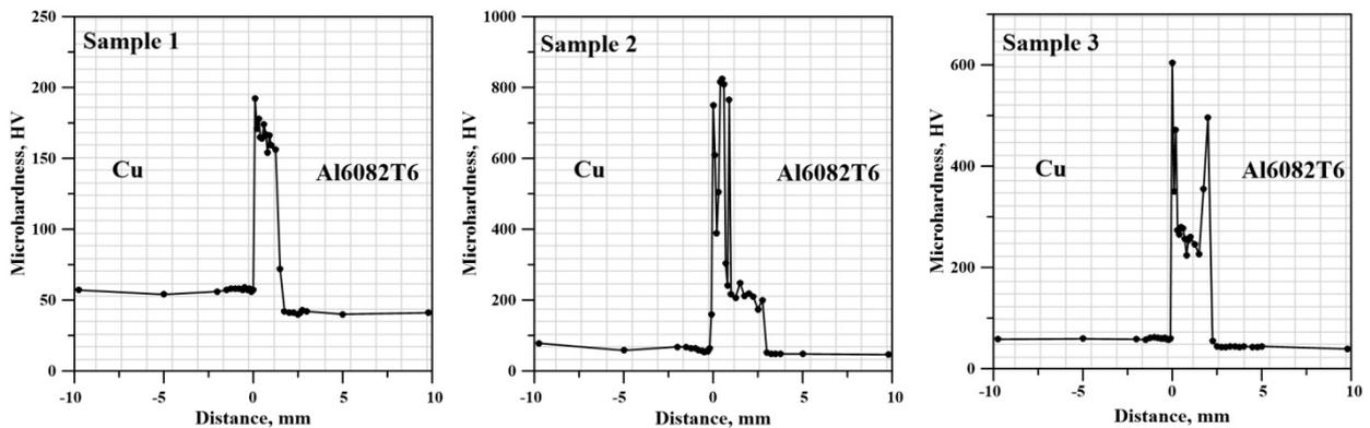
Fig. 5. Microhardness distributions of the weld formed using a beam power of: (a) 2400 W (sample 1); (b) 2700 W (sample 2); (c) 3000 W (sample 3)
