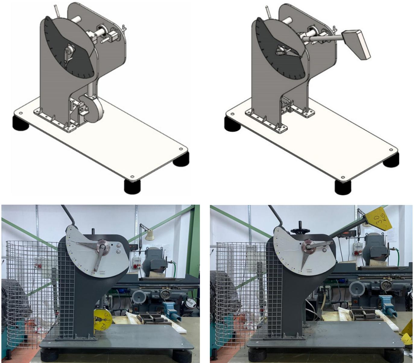
Fig. 1. Designed Charpy & Izod impact tester
