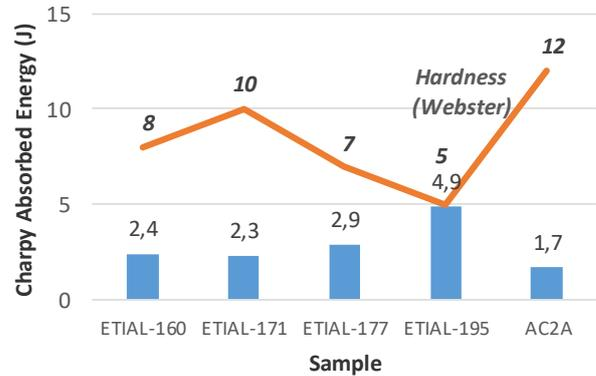
Fig. 6. Relation between absorbed impact energy and hardness
