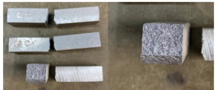
Fig. 7. Crack propagation in Charpy V-notch specimens
