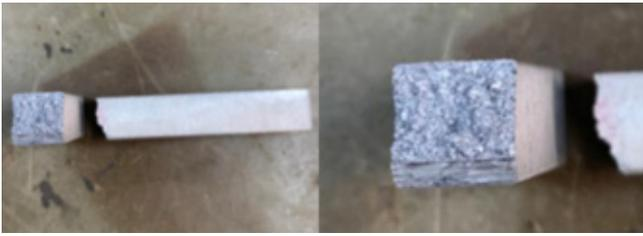
Fig. 9. Crack propagation in Izod V-notch specimens
