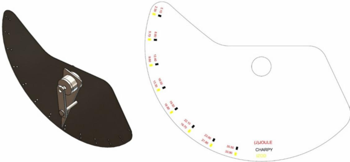
Fig. 2. Charpy & Izod impact energy indicator (J)
