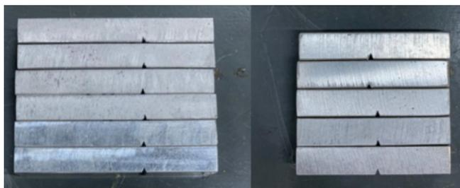
Fig. 4. Charpy and Izod test specimens
