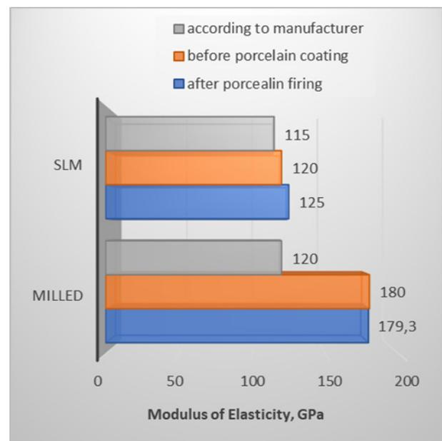
Fig. 5. Modulus of elasticity of Ti6Al4V alloy
