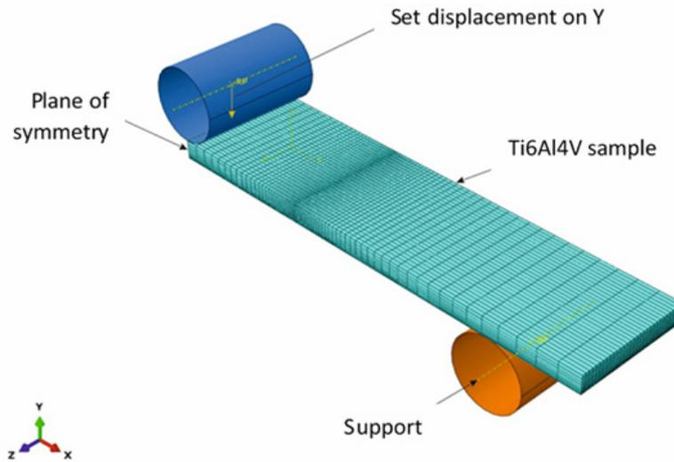
Fig. 3. FE model for determining the modulus of linear deformations of TiAl6V4 alloy
