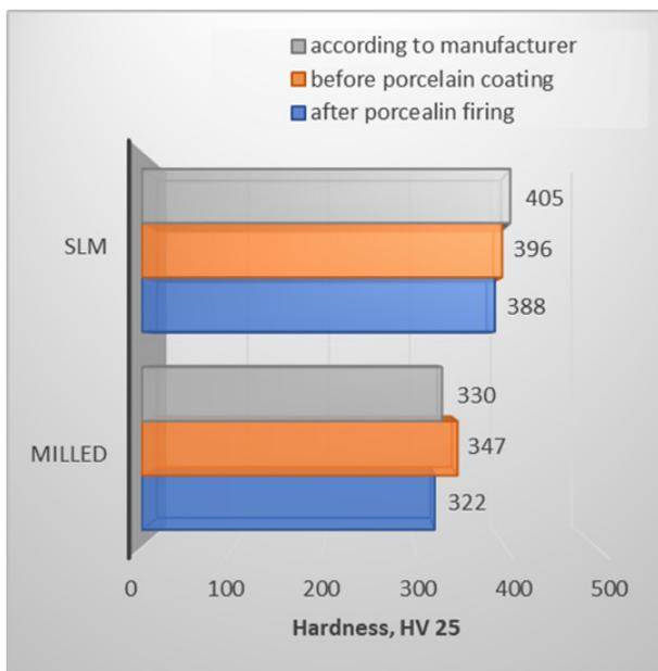
Fig. 4. Micro-hardness of Ti6Al4V alloy
