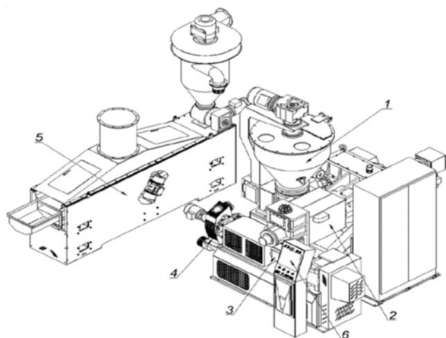
Fig. 2. System General View 1. Powder Feeding System 2. Main Rotor 3. Transfer Screw System 4. Pelletizer 5. Pellet Cooler Unit 6. Main Control Panel
