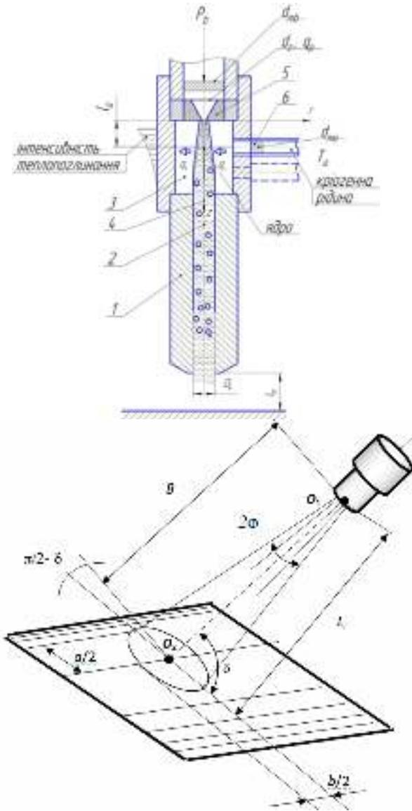
Fig. 1. The formation of a cutting water jet and its effect on the surface
