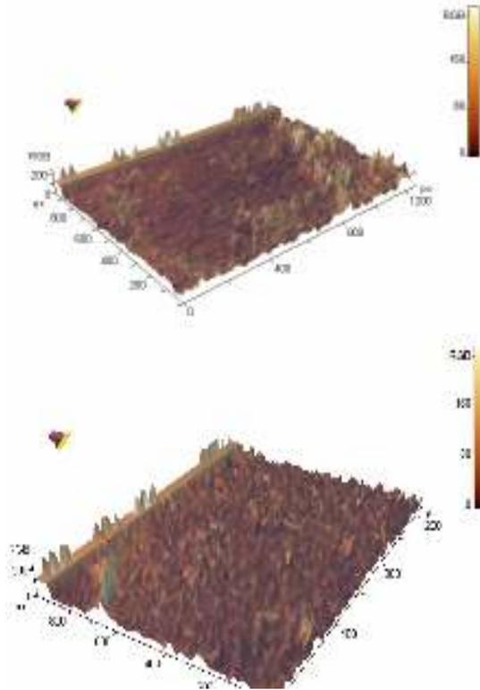
Fig. 4. Model of surface after cleaning water-ice flow
