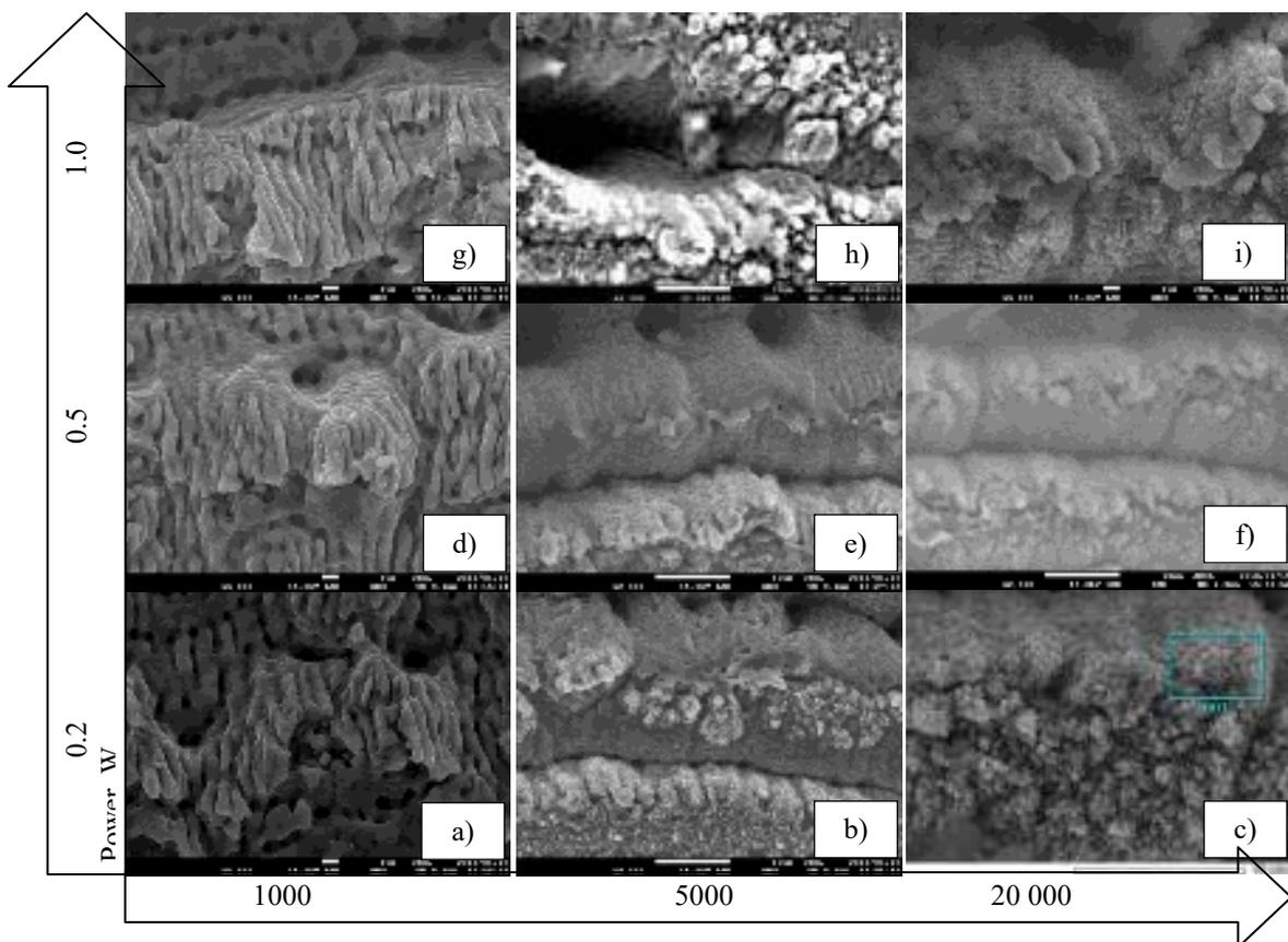
Fig. 5. Surface morphology of Ti6Al4V alloy after treatment with different regimes of picosecond laser (SEM images)
