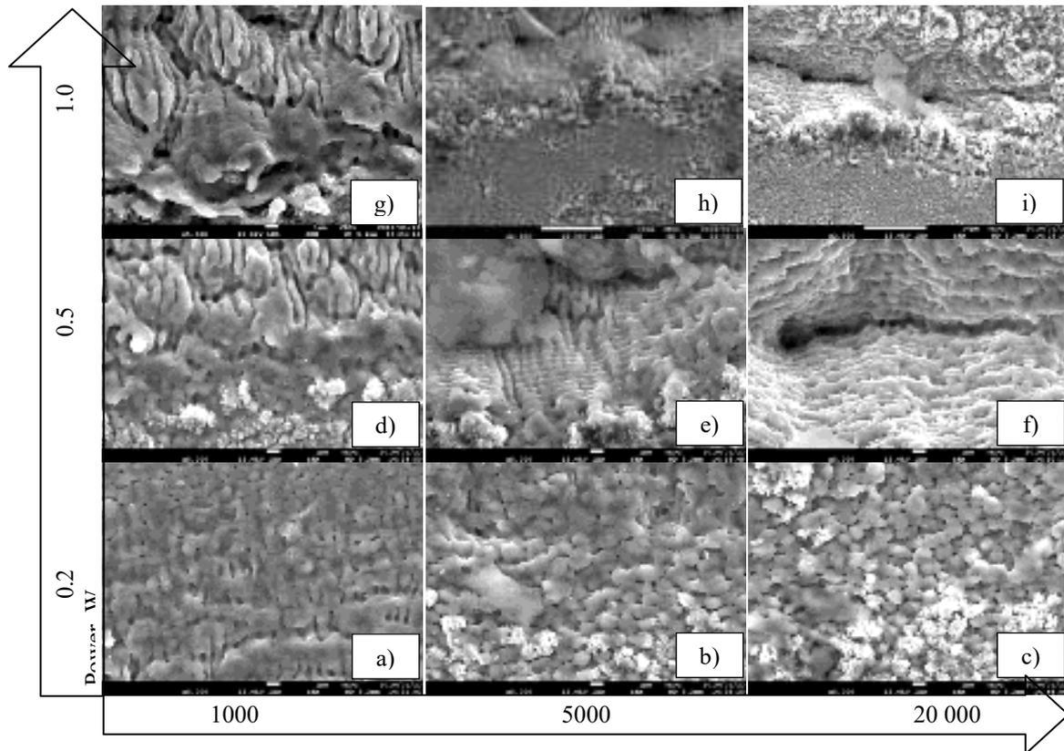
Fig. 4. Surface morphology of cpTi after treatment with different regimes of picosecond laser (SEM images)
