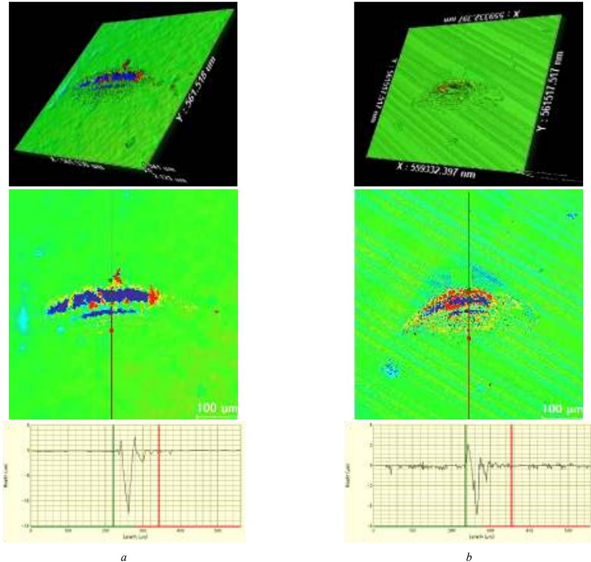
Fig. 3. 3D view, 2D view and cross section of the surface profile of cp Ti – a) and Ti6Al4V alloy – b), treated by picosecond laser (0.5 W and 20 000 pulses for cp Ti and 0.2 W and 1000 pulses for Ti6Al4V alloy.)
