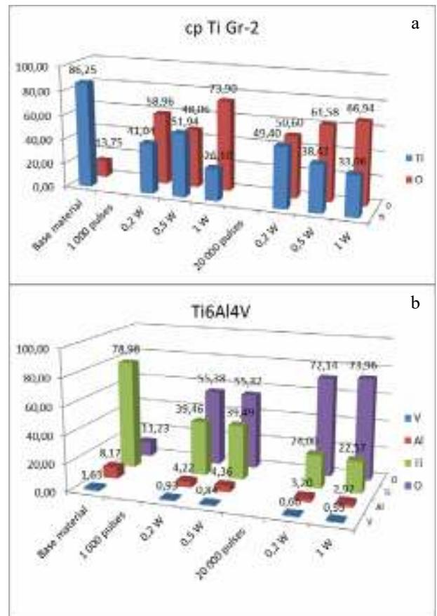
Fig. 7. Chemical elements distribution in the "melted zone" of cp Ti – a) and Ti6Al4V alloy – b), treated by picosecond laser with different regimes
