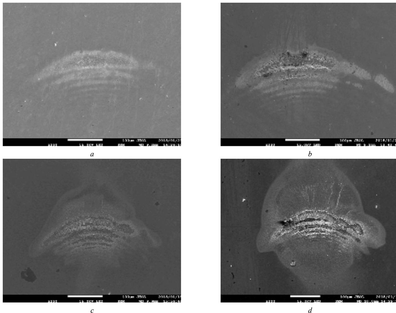
Fig. 2. Zones of laser influence on the surface of cp Ti (0.2 W, 1000 pulses – a) and 1 W, 5000 pulses – b) and Ti6Al4V alloy (0.2 W, 1000 pulses – c and 1 W, 1000 pulses – d) (SEM images)
