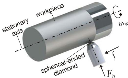
Fig. 2. Scheme of slide burnishing with spherical-ended tool
