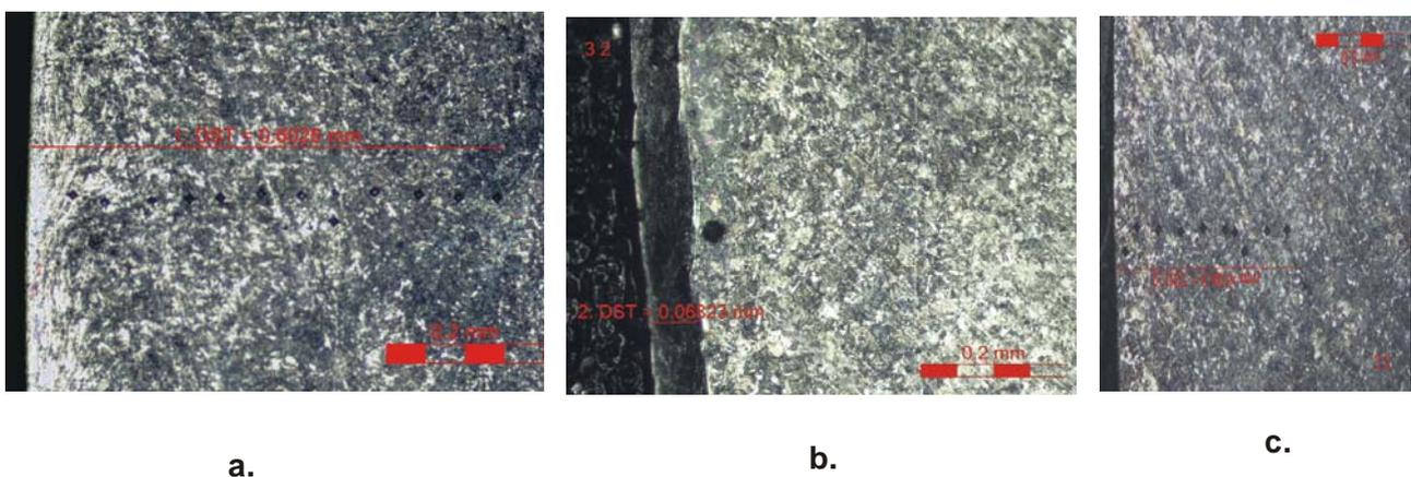
Fig. 5. Microstructure: a. after SB; b. after RB with  $F_b = 300N$ ; c. after RB with  $F_b = 1300N$
