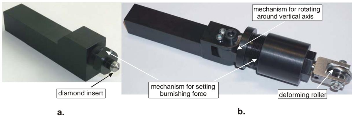
Fig. 3. Burnishing devices: a. diamond burnishing; b. single-roller burnishing
