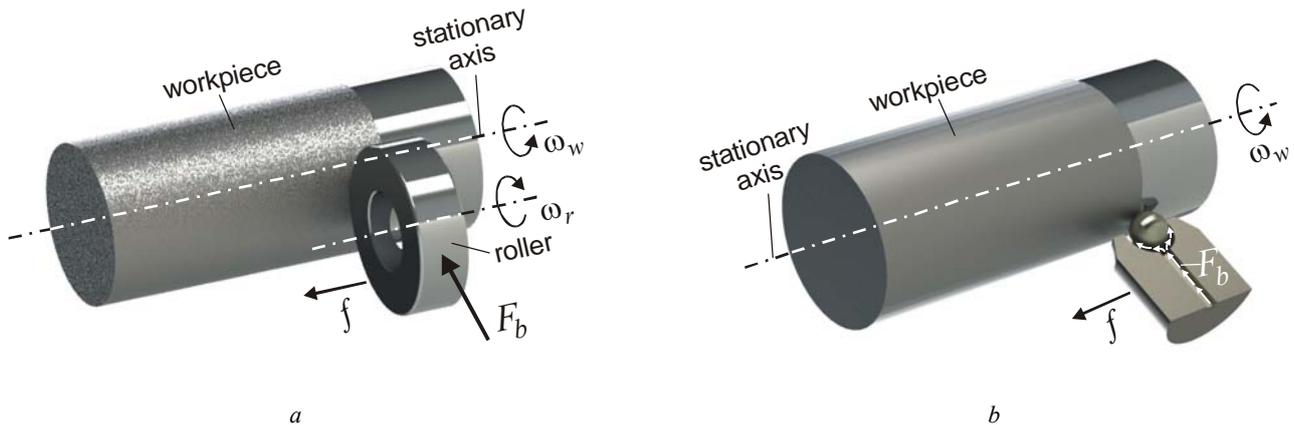
Fig. 1. Scheme of: a) single roller burnishing; b) ball burnishing with a hydrostatic sphere
