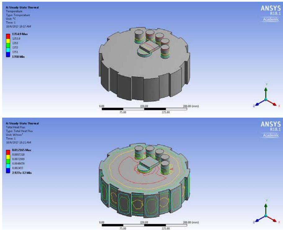
Fig. 2. Temperature fields and radiation of heated bodies in the chamber of vacuum furnace
