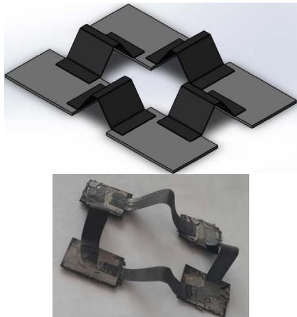
Fig. 3. Soldered structure from 4 plates of different thicknesses: 0,15 mm, 0,4 mm and 0,8 mm. The dimensions of the plates are 6×6 mm, the width of the connecting u-like tapes is 2,0 mm, the thickness of the tapes is 0,15 mm, the theoretical contact area is 7,0 mm<sup>2</sup>
