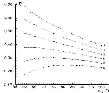
**Fig.2.** Dependence of the efficiency of the drying plant on the heating temperature of the drying agent in the solar collector ( $t_1$ ) and at the outlet from the drying chamber ( $t_2$ ): 1, 2, 3, 4, 5 and 6, respectively, at  $t_2=25; 30; 35; 40; 45$  and  $50^\circ\text{C}$
