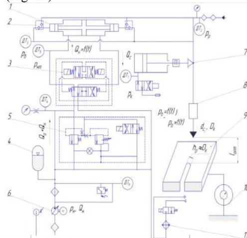
Figure 12 – Hydraulic system of the tested equipment with installed sensors
