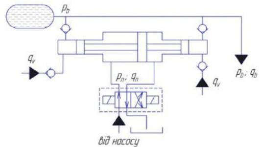
Figure 6 – Hydraulic system with a reverse multiplier
