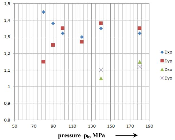
Figure 14 – Changing the shape and diameter of the hole while the pressure loss in the hydraulic system
