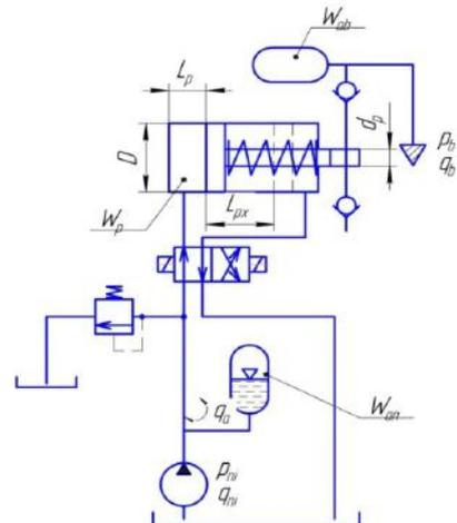
Figure 7 – Power supply system with single-sided multiplier
