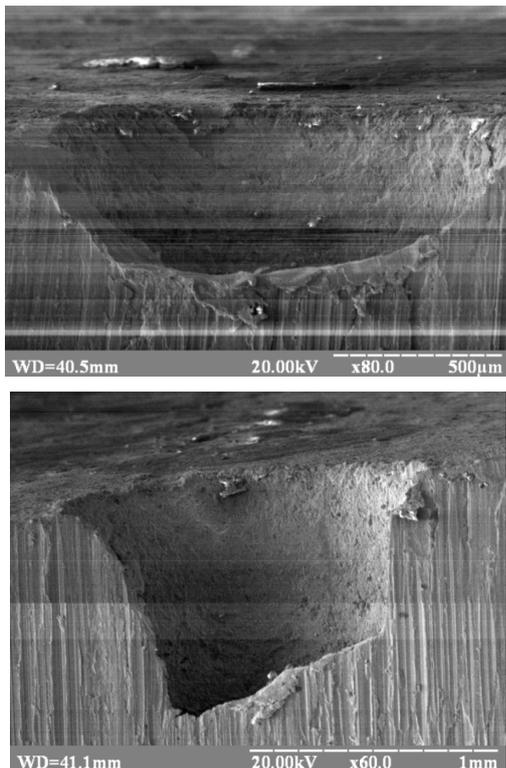
Figure 15– Microelectronic photographs of cross section of the cut while broaching the holes
