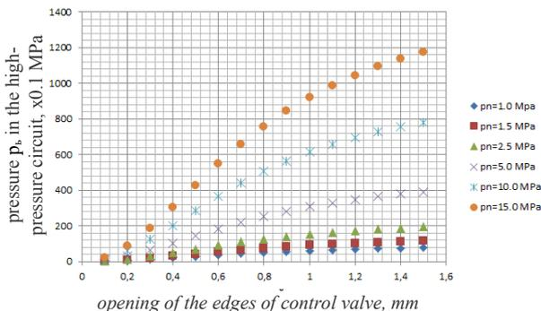
Figure 8 – Variation of pressure  $p_b$  in the high-pressure circuit while the openings of the edges of control valve, mm. Theoretical coefficient of multiplier  $K_{mp}=10$
