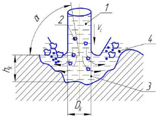
Figure 3 – Scheme of leakage hydroabrasive jet on the workpiece material:
