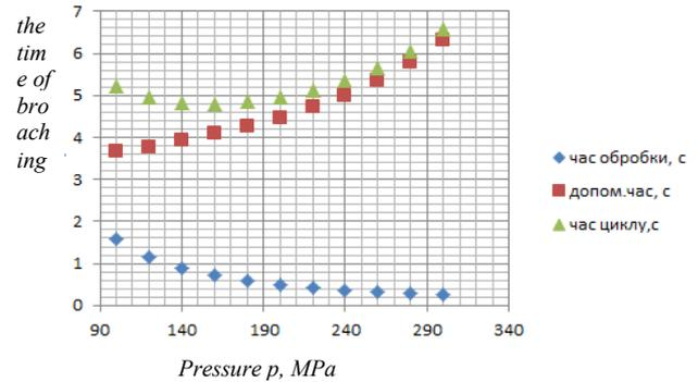
Figure 11 – Change in cycle time for different levels of fluid pressure in the high pressure circuit
