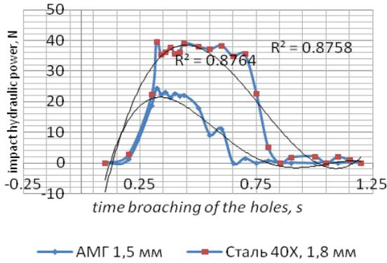
Figure 13 – Diagram of the change of efforts while broaching of the holes
