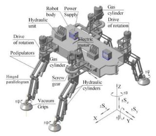
Fig.2. Walking mobile robot with energy accumulators
