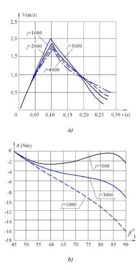
Fig.4. The effect of the rigidity j (N / m) of the elastic element on the speed (a) and the work performed by this element (b) in the second stage  $\beta_1 > 45^\circ$ , when the robot moves under the action of kinetic energy.
