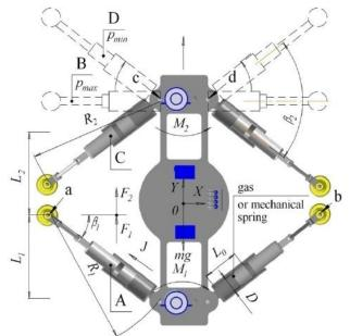
Fig.3. Scheme of the mobile robot (plan view)
