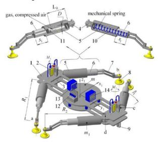
Fig.1. The robot model of arbitrary orientation with the accumulation and transformation of energy
