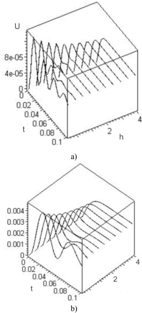
Fig.4. The time dependence of the system vibration amplitude depending on damping coefficient: a) - linear vibrations; b) - torsional vibrations
