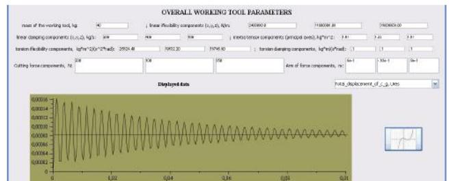
Fig.5. Determination of the stabilization time and the bar support system motions
