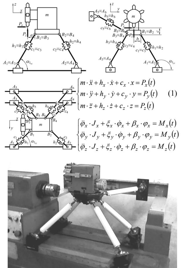
Fig. 2. The test bench for determining of the dynamic characteristics of the machine
