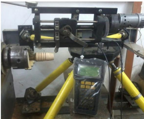
Fig.10. The vibration analyzer model 795M
