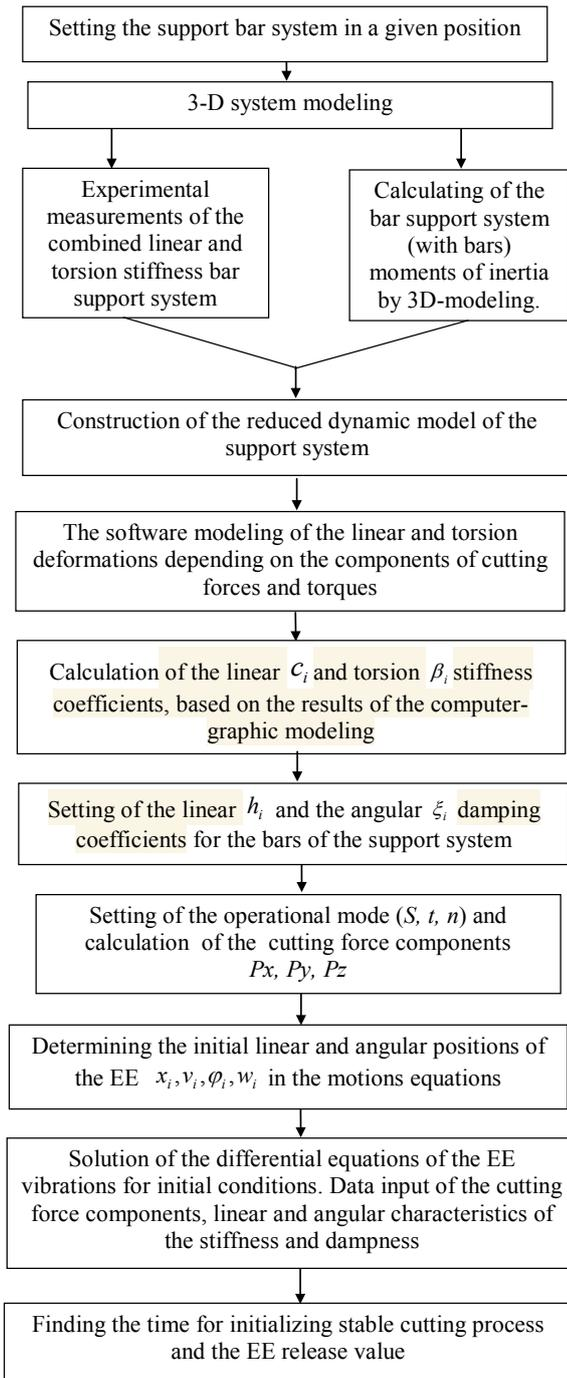
Fig. 1. The dynamic parameters determination sequence of the bar support system [5]
