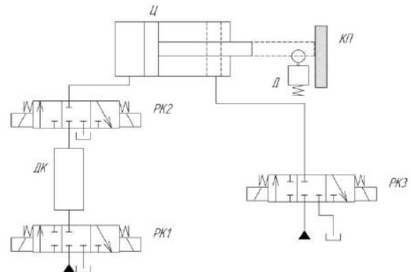
Fig. 1. Diagram of the actuator positioning
