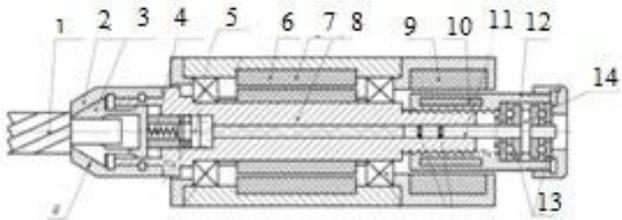
Figure 5 - Longitudinal section of the spindle-motor assembly
