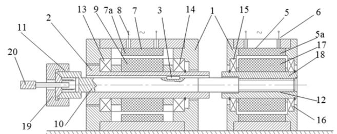
Figure 7 - Longitudinal section of the spindle-motor assembly
