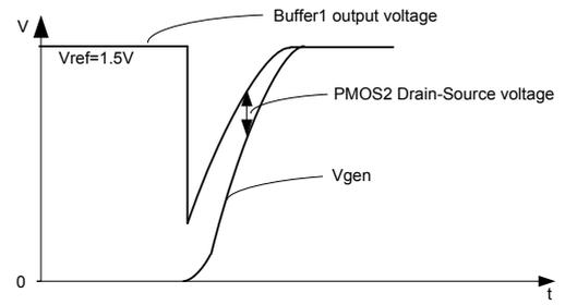
Fig. 4.  $V_{gen}$  transition when rising slope occurs
