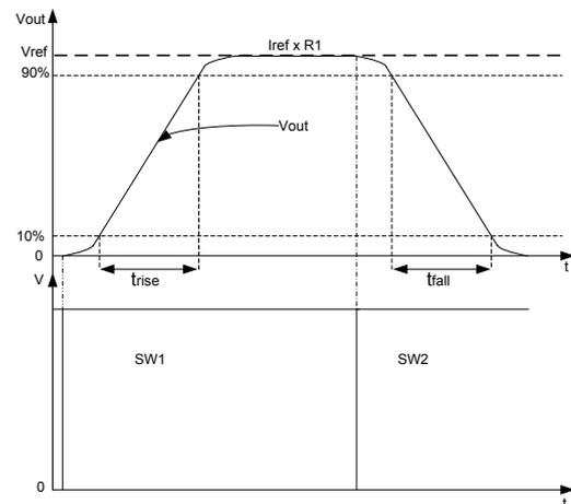
Fig. 2. Generated voltage output pulse and digital control signals
