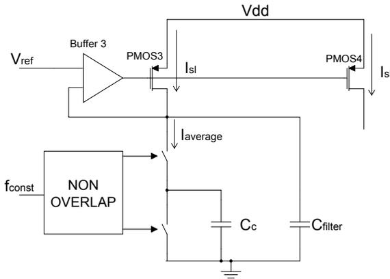
Fig. 3. Circuit used for  $I_{sl}$  generation
