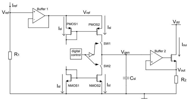
Fig. 1. Generator of current slopes
