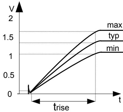
Fig. 5.  $V_{gen}$  transition when rising slope occurs
