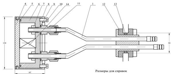
**Fig. 4.** The design of the worked out device magnetron sputtering with a disk cathode, diameter of 130 mm
