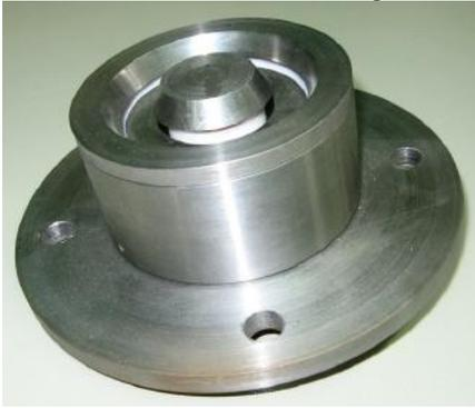
**Fig. 2.** Photo of ion source with a cold cathode
