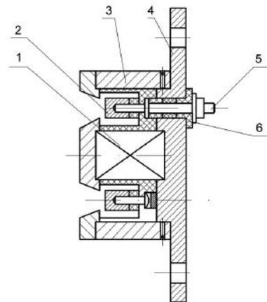
**Fig. 1.** The ion source with a cold cathode and a divergent flow of plasma gas discharge
