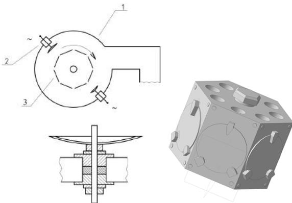
**Fig. 3.** The discharge electrodes in a vacuum working chamber and accessories. 1 - working chamber, 2 - electrodes, 3 - treated objects
